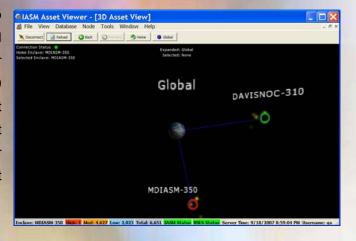
The Promia Asset Viewer uses a "warp" effect (shown in the picture to the right) as its unique visual cue that an operator is navigating from the Global View to a remote Promia Raven 1100 appliance. During the "warp" the AV logs into the remote device to retrieve its asset and incident information for display in the usual fashion. The "warp" capability thus enables any combination of distributed or centralized network security operations management.
